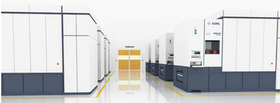
When it was launched in 2000, the TWINSKAN lithography platform caused a revolution. Today, it is the de facto standard for volume manufacturing on 300-mm wafers. Its unique dual-stage design allows non-stop parallel processing: measuring one wafer while imaging another for maximum accuracy and productivity.
