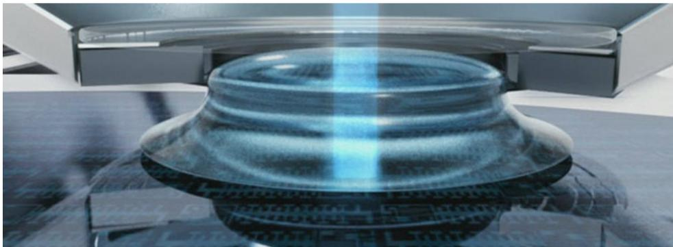
Both systems push water-based immersion to its limits. Their hyper NA of 1.35 delivers unrivalled depth of focus and resolution, enabling high-yield manufacturing at smaller nodes than ever before.
